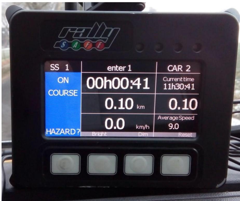
'ON COURSE' means you have started the Regularity/Test, not necessarily that you are on the right route ;-). Also the time since the start is indicated (here 0h00:41 = 00:00:41), the distance, the distance since the last Reset and your actual speed. (The Average speed will not be shown or will be deliberately unreliable!). The unit is in Stage/Safety mode now and will warn you (and other competitors) for potentially unsafe situations.
